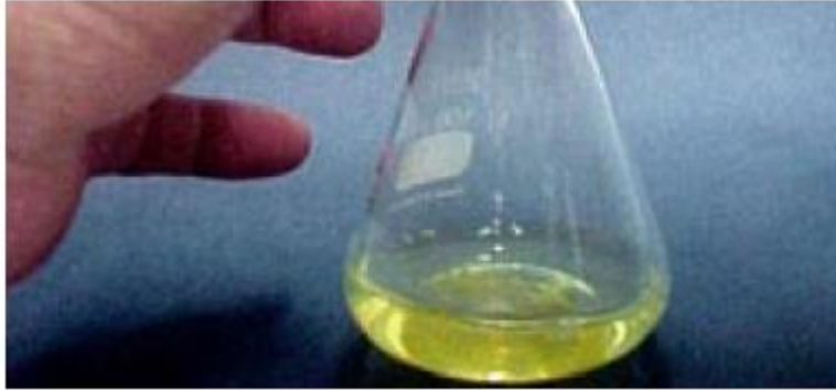
Figure 1 Before the addition of any silver nitrate the chromate indicator gives the clear solution a lemon-yellow color.
