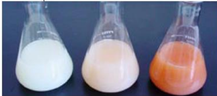
Figure 2: Left flask: before the titration endpoint, addition of \text{Ag}^+ ions leads to formation of silver chloride precipitate, making the solution cloudy. The chromate indicator gives a faint lemon-yellow color. Centre flask: at the endpoint, all the \text{Cl}^- ions have precipitated. The slightest excess of \text{Ag}^+ precipitates with the chromate indicator giving a slight red brown coloration. Right flask: If addition of \text{Ag}^+ is continued past the endpoint, further silver chromate precipitate is formed and a stronger red brown color result. NB: The titration should be stopped
