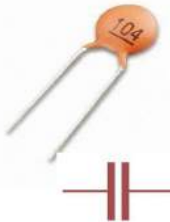
Non-Polarized Ceramic Capacitor and its electric Symbol
