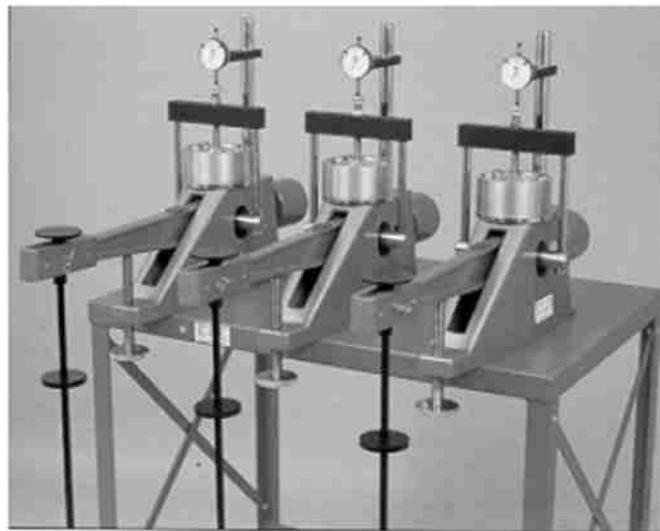
Figure 9:1 - Consolidation frame with Dial Gauge (with three gangs)
