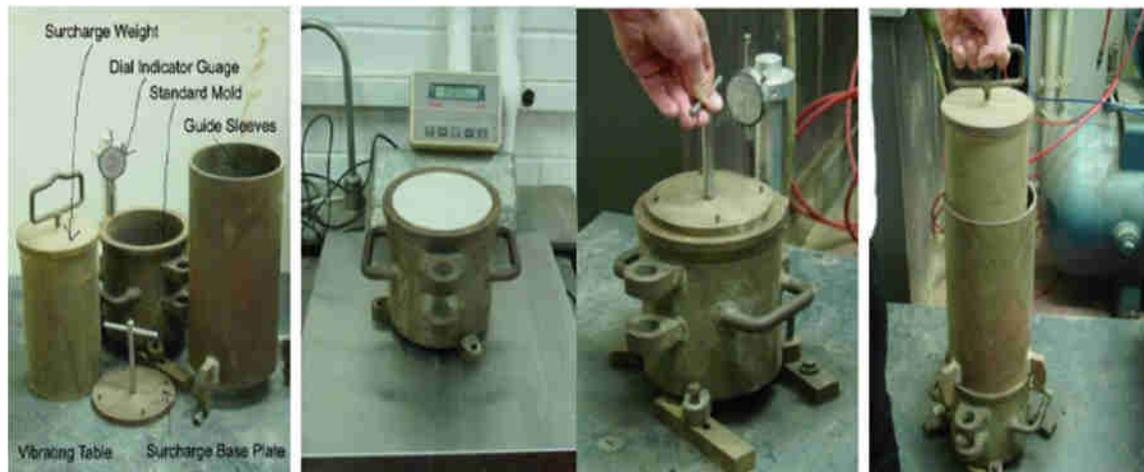
Figure 4:1: Relative density of soil determination apparatus
